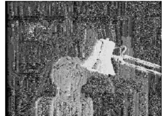
The disparity map is very noisy, due to a low signal-to-noise ratio (SNR).
