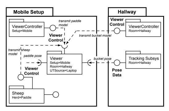
Figure 7.11: DWARF components involved in runtime reconfiguration of the mobile setup's Viewer. This UML diagram shows the system state in location Hallway.
