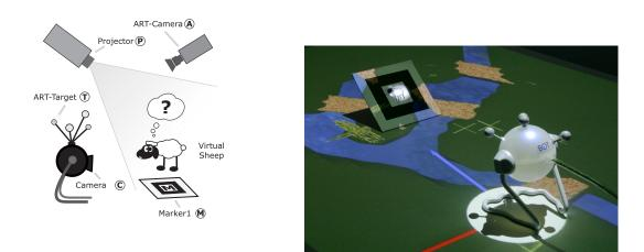
Figure 3.10: Extended tracker range setup: An ART system tracks a camera that detects a fiducial marker outside the ART system's range. This information gets used to project a virtual sheep onto the marker.
