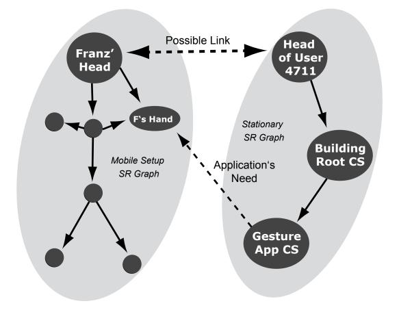
Figure 6.6: Two SR graphs of a mobile setup and a stationary environment. The graphs should be connected by adding an edge between the nodes *Franz' Head* and *Head of User 4711*.
