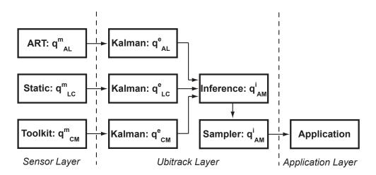
Figure 5.7: DWARF data flow components of extended tracker range example. The diagram shows the SR graph functions corresponding to the individual services and the logical layering of the services. Arrows indicate the data flow.
