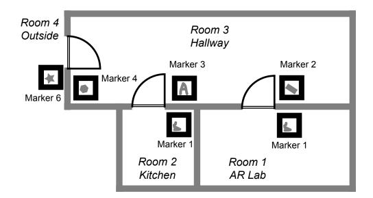
Figure 6.4: Physical setup of ARCHIE scenario. Note that the ARToolkit markers used for spatial indexing can be reused, the outgoing marker both in the ARLab and the kitchen are identical.
