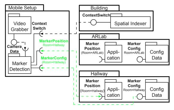
Figure 6.3: Example setup after configuration change. The marker detection service changed its ability attributes and need predicates such that it gets a new configuration from the hallway's corresponding service and sends its data to another application.
