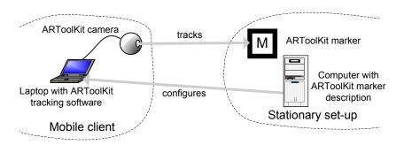
Figure 6.7: A stationary locatable is to be identified by a mobile camera. Thus, the stationary environment has to transmit information about the locatable to the mobile setup. (Taken from [114].)
