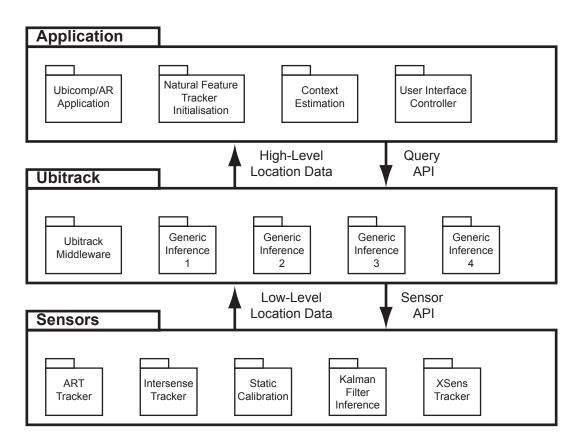
Figure 5.5: Layered Ubitrack architecture. The Ubitrack layer is an abstraction from the low-level location sensors and provides a powerful API to arbitrary applications.
