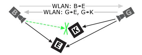
Figure 3.12: Shared optical tracking setup: Two cameras try to detect the pose of two markers. Missing information is exchanged over a wireless network.
