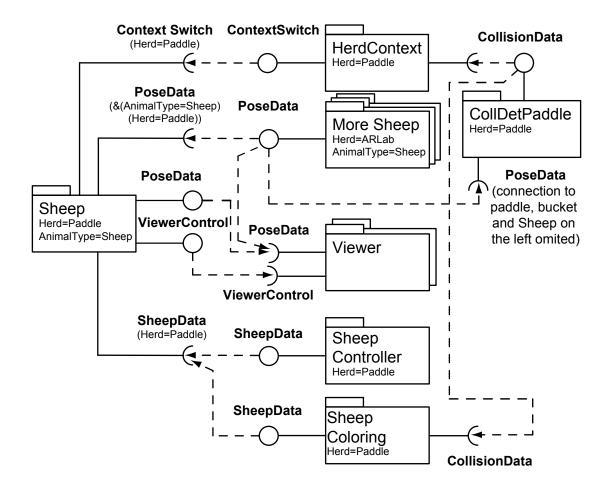
Figure 7.13: DWARF components involved in runtime virtual sheep reconfiguration if the sheep is in herd state Paddle.
