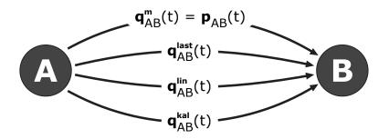
Figure 3.4: Inference Graph  $G(\Psi)$ : An individual edge is added for every inference of the spatial relationship between objects represented by two nodes.
