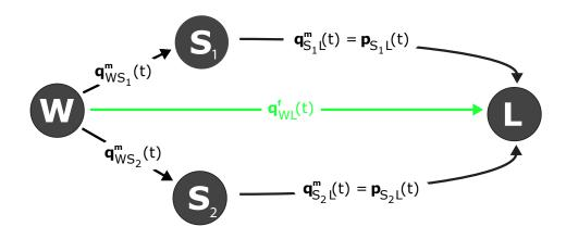
Figure 3.9: Modeling complementary sensor fusion in the Ubitrack formalism.
