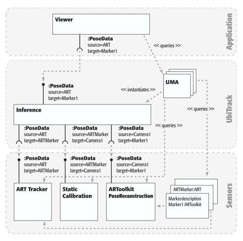
Figure 5.8: UML diagram of the DWARF-based implementation of the extended tracker range scenario.
