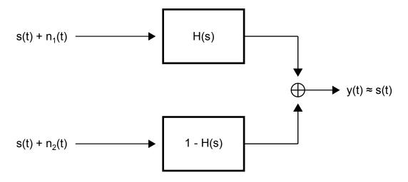
Figure 2.1: A complementary filter for two measurements (taken from [11]).
