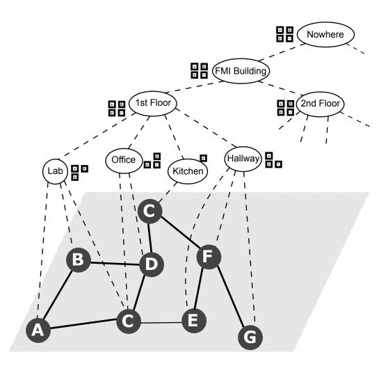
Figure 6.9: Hierarchical reduction of configuration data. At every hierarchical step, new sets of object descriptions are used.
