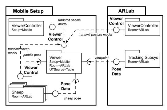
Figure 7.10: DWARF components involved in runtime reconfiguration of the mobile setup's Viewer. This UML diagram shows the system state in location ARLab.
