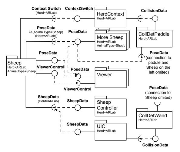
Figure 7.12: DWARF components involved in runtime virtual sheep reconfiguration if the sheep is in herd state ARLab or Monitor.
