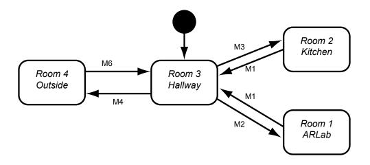
Figure 6.5: State transition diagram of ARCHIE spatial indexer.
