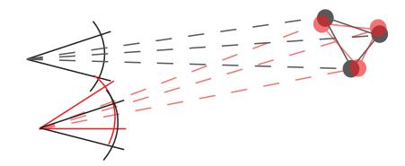
Figure 3.1: Why the SR graph needs to be directed: If the object's real state (black) is measured with some error (red), the positional accuracy remains high, while the orientational accuracy degrades. If we look at the situation from the object's perspective and want to estimate the camera's pose in the object's coordinate system, the positional accuracy degrades, while the orientational accuracy is high.
