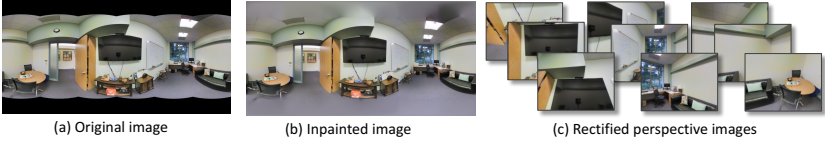
Fig. 6. Example of equirectangular image with/without inpainting and extracted rectified perspective images.
