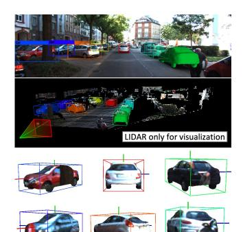
Figure 1. Top (from left to right): our 2D detections, 3D boxes, and meshed shapes inferred from a single monocular image in one forward pass. Middle: our predictions on top of a LIDAR point cloud, demonstrating metric accuracy. Bottom: example well-localized, metrically-accurate, textured meshes predicted by our network.
