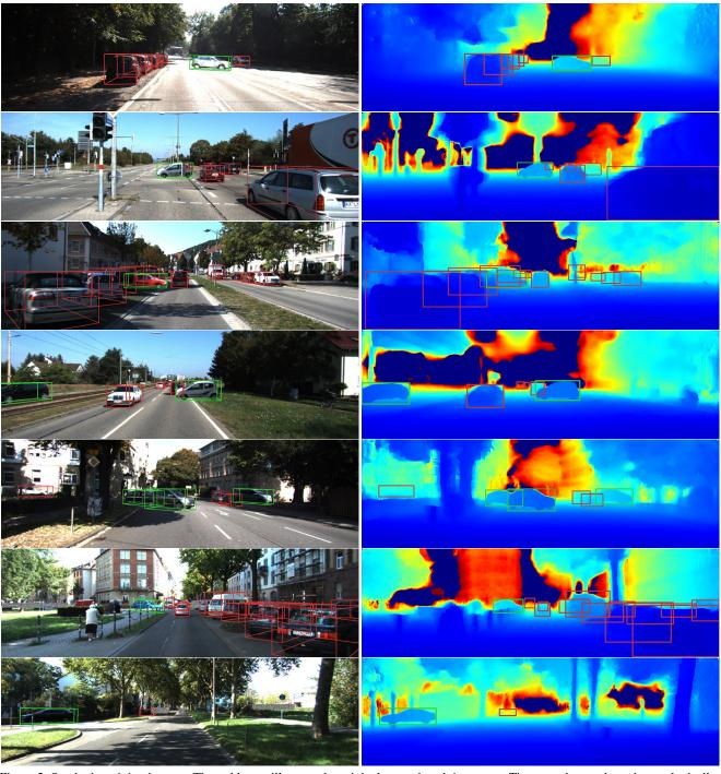
Figure 2. Synthetic training images. The red boxes illustrate the original ground truth instances. The green boxes show the synthetically-added data via rendering random instances from our generated car collection in new poses. The noisy patterns in some images enforce 'ignore'-annotated parts of the image to not be used by negative mining during training.
