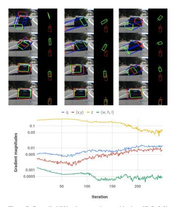
Figure 7. Controlled lifting loss experiment with given 2D RoI  $\mathcal X$  over multiple runs with different seeding. Top: Visualizing  $\mathcal F(\mathcal X)$  during optimization in camera and bird's eye view. Bottom: Gradient magnitudes of each lifting component, averaged over all runs. We refer to the supplement for the full animations.
