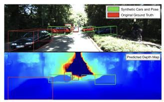
Figure 6. Synthetically generated training sample. Top: Green bounding boxes show original ground truth cars and poses. In contrast, red boxes illustrate the rendered meshes from a sampled 6D pose. Bottom: Augmented depth map from SuperDepth [33]. Notice that we utilized the annotated meshes, which we colored using the ground truth pose and our projective texturing.
