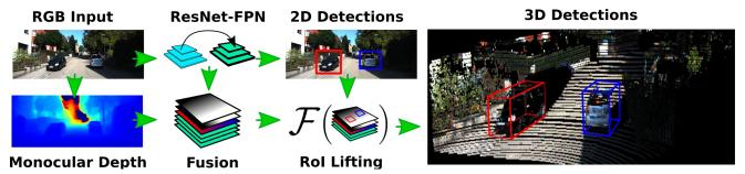
Figure 2. We process our input image with a ResNet-FPN architecture for 2D detection and a monocular depth prediction network. We use the predicted Regions of Interest (RoI) to extract fused feature maps from the ResNet-FPN and depth network via a RoIAlign operation before regressing 3D bounding boxes, a process we call RoI lifting.
