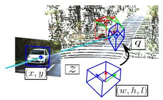
Figure 3. Our lifting  $\mathcal{F}$  regresses all components to estimate a 3D box  $\mathcal{B}$  (blue). From here, our loss minimizes the pointwise distances towards the ground truth  $\mathcal{B}^*$  (red). We visualize three of the eight correspondences in green.
