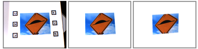
Figure 6: The steps taken to prepare an image for evaluation: Left the captured image, in the middle the undistorted image with the background removed, on the right the final image with randomized borders.
